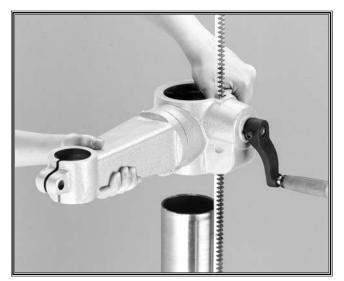
Figure 11. Correct rack orientation.
